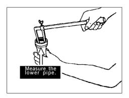
[7]Measure the inner diameter of lower pipe of front shock absorber with callipers.Check whether it exceeds the limit value of maintenance.Replace it if exceeds.
