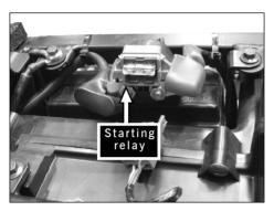
[3]Check whether starting relay is in good working condition.Replace it with the same type if it is not in good working condition.
