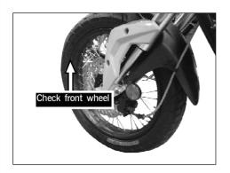
[2]If front wheel is deformed by stricking or vibration, so that the bike run out of way or steering control trembling or vibrating. The wheel need to be replaced or adjusted.
