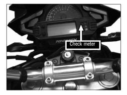
[3]Check whether the connection of speedometer is looseness.
