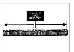
[8] Remove the returning spring of front shock absorber and check its abrasion. Replace it if worn.
