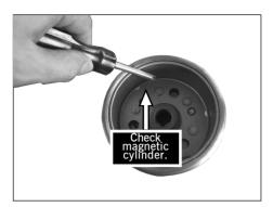
[5]Check whether the magnetic cylinder of generator rotor fades magnet.Replace magnetic cylinder if fades.
