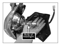
[1]Dismantle the cover of headlight and check whether the holder and bulb are in good working condition. Remove the bulb and check whether it is burnedout.Replace it with the same type if burned-out. Bulb type: HS1 12V 35/35W
