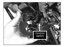
[4]Dismantle the switches of left and right controls. Check whether they are damaged or have short circuit.Repair or replace them if have problems.
