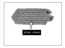
[5]Dismantle the spring clamp of drive chain. Remove tie-in of drive chain and drive chain.Check the abrasion of the tie-in of drive chain and replace it if necessary.
