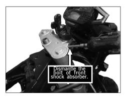
[1]Check the effective stroke and performance of front shock absorber, and check whether there is leakage from front shock absorber.
