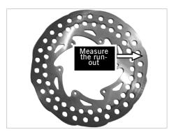
[15]Measure the run-out of brake disc by dial indicator and the limit value is 0.3mm.
