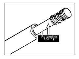
[5]Dismantle front shock absorber pole and lower pipe. Check their abrasion.Replace them if worn.
