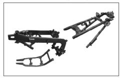
The frame of this motorcycle adopts pipe jointing and crooked girder. It has high intensity, good firmness and good suitability. It mainly consists of head pipe, main frame, tail pipe, rear supporting pipe and low bending pipe. It is made through the methods of jointing, riveting and so on.
