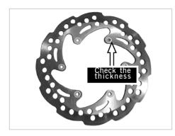
[7]Measure the thickness of front brake disc with micrometer. The limit value of repair is 2.0mm.
