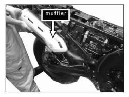
[3]Remove the seal gasket of muffler and check whether the gasket is damaged.Replace it if damaged.
