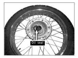
[9] Remove the rear drive sprocket and check it for wear.
