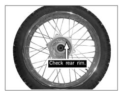
[10]Dismantle the locknut of rear axle .Remove rear axle and rear wheel assembly.
