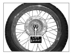
[8]Remove the oil seal of cushion body of rear drive sprocket wheel and check its abrasion.
