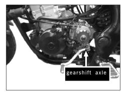
[2]Dismantle bolts of left rear cover of left crankcaseand remove left rear cover of left crankcase.
