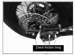
[13]Disassemble the fixed bolt of brake disc and remove it.
