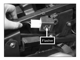
[2]Remove the flasher socket of signal system and measure the flasher with multimeter.Check whether it has short circuit.Replace it if short circuit.
