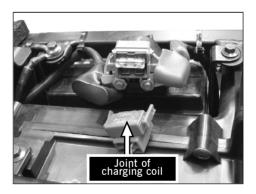
[4]Remove left cover of engine and the stator of generator.Measure the resistance of generator stator with multimeter and check whether the resistance has short circuit or open circuit.Replace it if short or open circuit. Resistance Value
