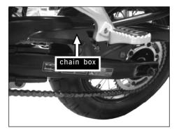
[3]Check the abrasion of small drive chain and replace the chain assembly if necessary.
