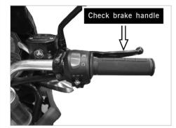
[1]Hold front brake control with right hand to check the brake performance of front brake. The standard free stroke is:  $10 \text{mm} \sim 20 \text{mm}$
