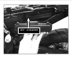
**3** Disassembly and Maintenance of Intake System [1]Dismantle suspension bolt of air cleaner and clamp screw of inlet pipe.Remove air cleaner assembly.
