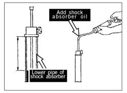
[9]When installing front shock absorber,add front shock absorber oil according to the stated.The standard volume of front shock absorber is (330  $\pm$  5)mL.
