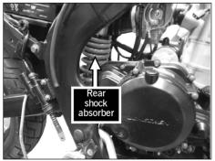
[1]Check whether the spring of rear shock absorber becomes soft and its damper has leakage.Replace shock absorber assembly if the rear damper has leakage.
